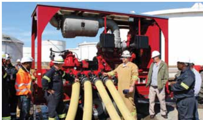
The Williams Dependapower DPPAT-6040-CAT-R-T3 draft pump
