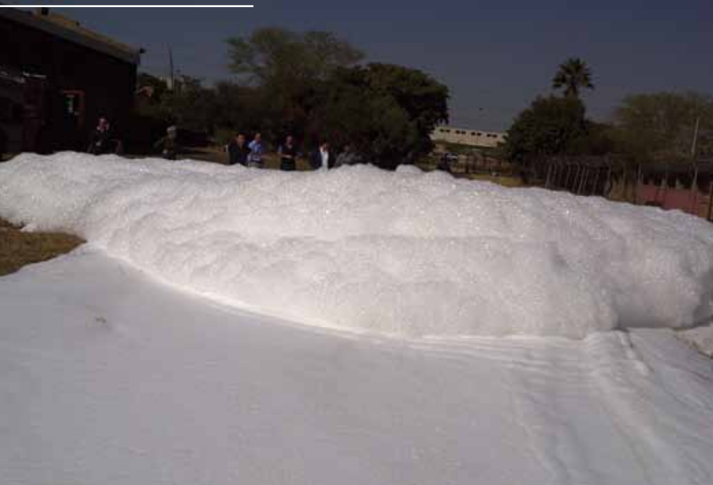
A demonstration done in South Africa through a Turbex as a high-expansion foam
